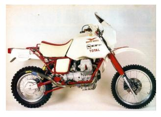
The main alteration from the prototype design for the competing Dakar bikes was fitting an additional 12 litre fuel tank in the seat area to meet the Dakar's '50 litres of fuel' requirement. The rear of the frame also changed substantially to support relocated electrical components and the mandatory 2 litres of water. The power output was around 62 HP and dry weight of 162 kilograms, which was similar to the Cagiva Elefant. The full Titanium exhaust system contributed to the low weight.
